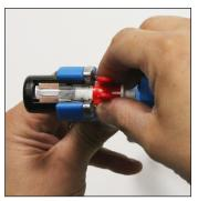
1. Remove a TSU punch from the packaging. Punches should be assembled as one piece; if they have come apart, reassemble. Align the groove of the punch with the chamber at the base of the applicator.
