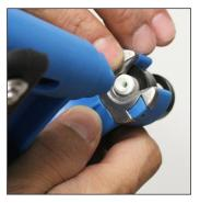
3. Remove the red plastic clip by pulling it outward. Be careful as the metal cutter above the clip is very sharp. Ensure the applicator is loaded with an unused green punch (if the red plunger is visible, the punch is used and should be replaced with one that is unused).
