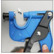
5. Reopen the chamber and remove the punch from the applicator. Check that sampling has been successful (red plunger is visible, sample is in fluid in punch). Remove the used cutter from the applicator by pulling the handles apart. Discard carefully as the cutter is very sharp.
